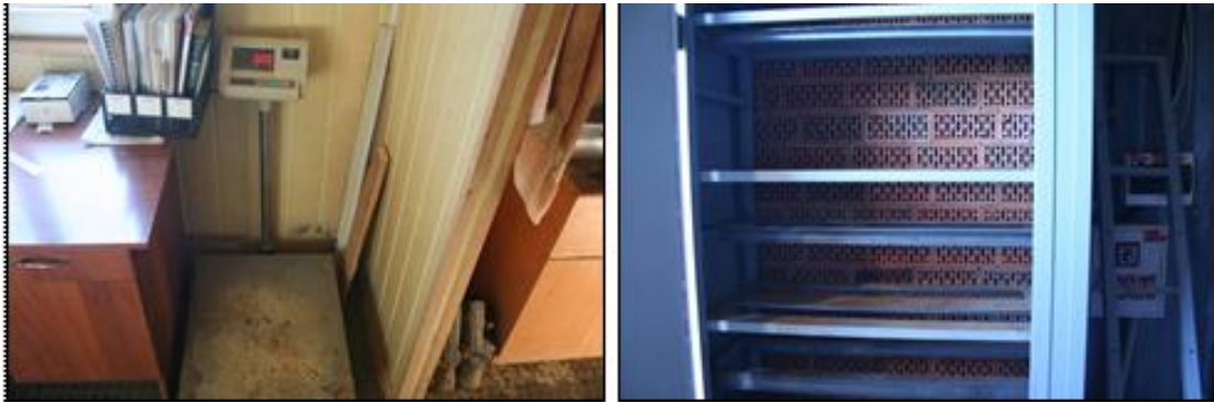
Figure 4-6: Scale Balances for Weighing Received Samples and Dewatering Box
