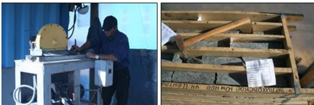
Figure 4-4: Core Sawing and Sampling
